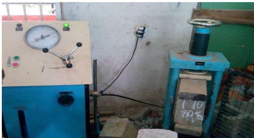
Plate 3: Compressive testing of the developed Sandcrete
