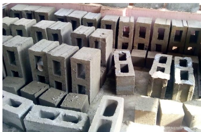
Plate 2: Sandcrete block and cube during the curing process
