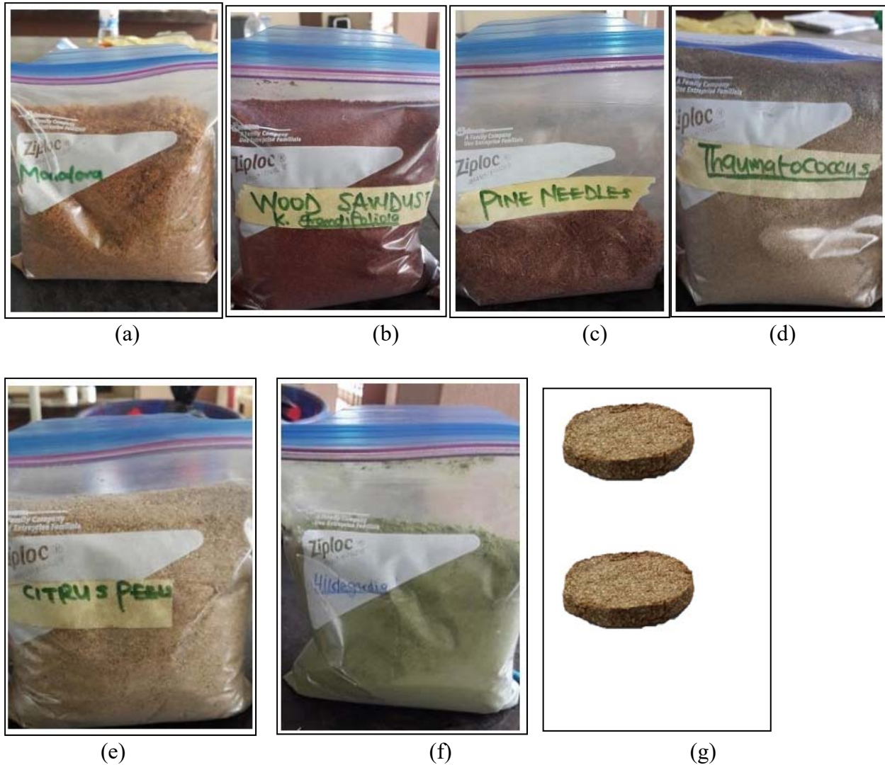
Plate 1: Pulverised tinder samples used for the lighter production: (a) Monodora myristica seeds, (b) Khaya grandifoliola sawdust, (c) Pinus caribaea needles, (d) Thaumatococcus daniellii leaves, (e) Citrus sinensis peels, (f) Hildegardia barteri leaves, (g) solid charcoal lighter produced
